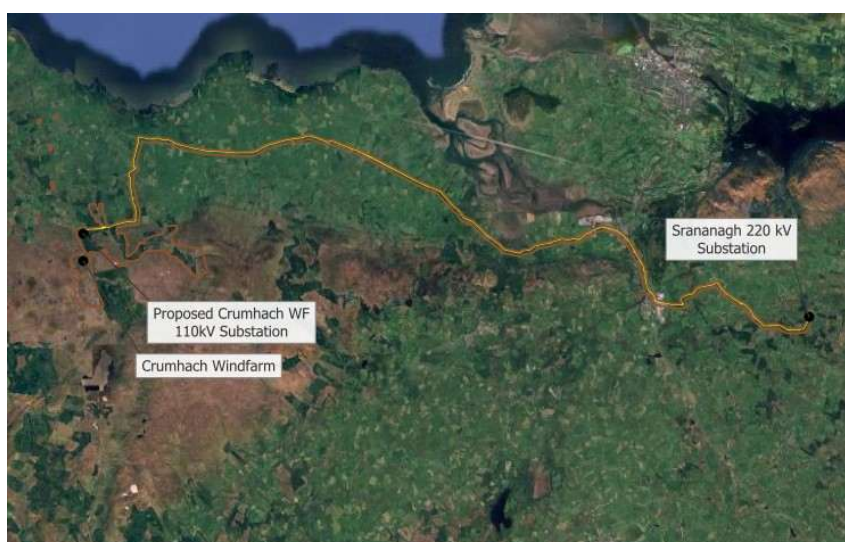
Figure 1: Grid Connection Route Layout Plan
